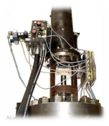
The hydraulic aggregate feeds to the hydraulic cylinders on the HP/LP bypass valves and the hydraulic cylinders on the corresponding spray water control valves.
